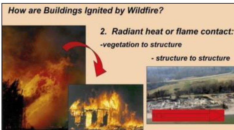
Figure 8. Radiant heat and flame contact allows fire to spread from vegetation to structure or from structure to structure.
